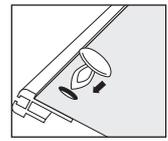
Maximum security. Carefully make holes in the banner to align with the holes in the rail. Insert the plastic push pins provided.
