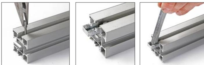
**3.** Replace the pin. Mount the pivot and the lever.
