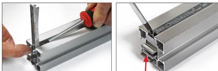
**4.** Push the lever back into the channel and push down the pin and gently tap the pivot to put back into place. Replace the small screw with a new one. Press the Clamp upward when fastening the screw.
