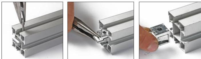
**2.** Remove the pin first, followed by the clamp. Replace the clamp, with the larger hole facing up.
