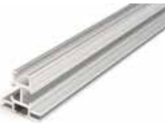
Fabric profile, half Total size: 37 x 37 x 3300 mm Weight: 3234 grams (980 g/m) Item IS-9330
