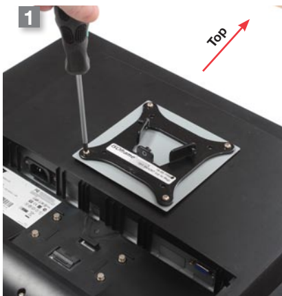
Attach the holder to the LCD
