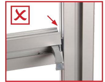
Wrong – not square
