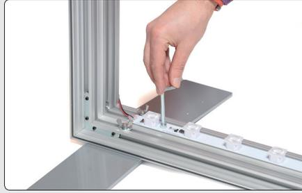
**2** Lock the two screws with the Allen-key.
