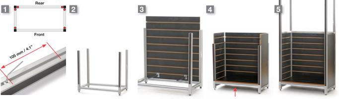
First determine the desired height for the bottom shelf. Install the stop screws on the base posts so that the top edge of the stop screw is 105mm/4.1 inches below desired shelf height.
